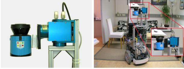
Figure 9. Tilting laser range scanner for capturing the test data.
