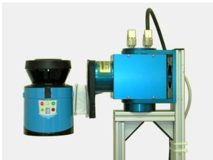
Fig. 7. Tilting laser range scanner for capturing the test data
